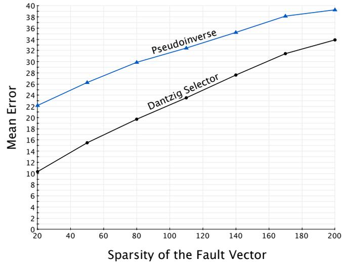
Fig. 2. The mean error between the reconstructed fault vector and the real fault vector for different sparsities of the fault vector using two different methods ( $\|\mathbf{f} - \mathbf{f}^*\|$  and  $\|\mathbf{f} - \mathbf{f}_p\|$ ).
